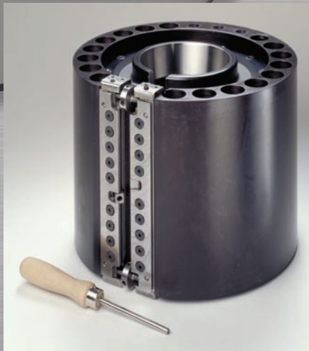
Speed clamp cylinders for waterless plates
